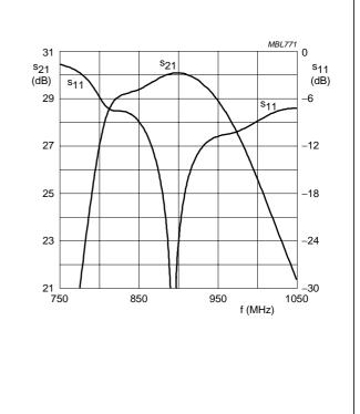
Fig.11 s-parameters as a function of frequency.
