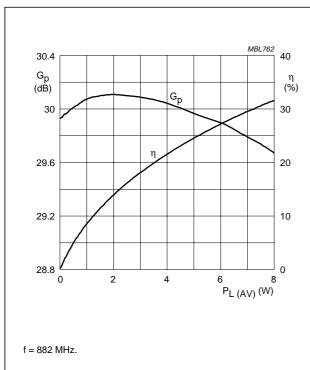
Fig.2 IS95 power gain and efficiency as functions of load power; typical values.
